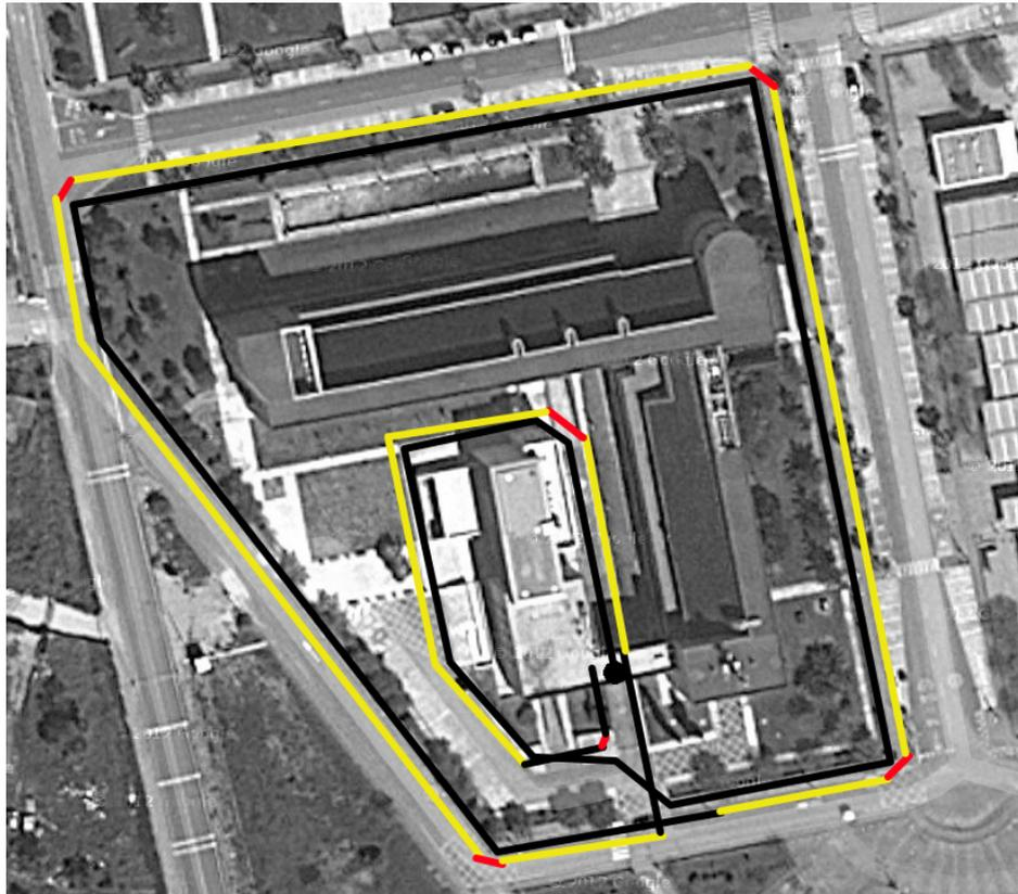
Figure 10: Path followed by the camera during the UIB large loop experiment. The black point indicates the beginning of the sequence, the black lines show no loop closure detections (highest posterior probability is under  $T_{loop}$ ), the red lines show rejected hypotheses (no epipolar geometry is satisfied) and the yellow lines represent loop closure detections (highest probability is above  $T_{loop}$  and the epipolar constraint is satisfied).
