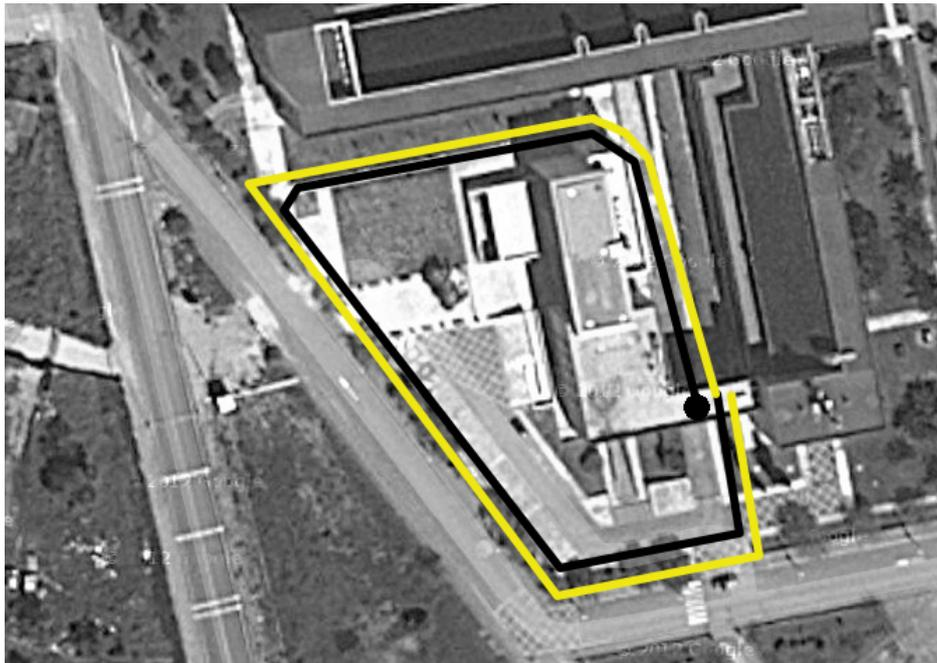
Figure 8: Path followed by the camera during the UIB small loop experiment. The black point indicates the beginning of the sequence, the black lines show no loop closure detections (highest posterior probability is under  $T_{loop}$ ) and the yellow lines represent loop closure detections (highest probability is above  $T_{loop}$  and the epipolar constraint is satisfied).
