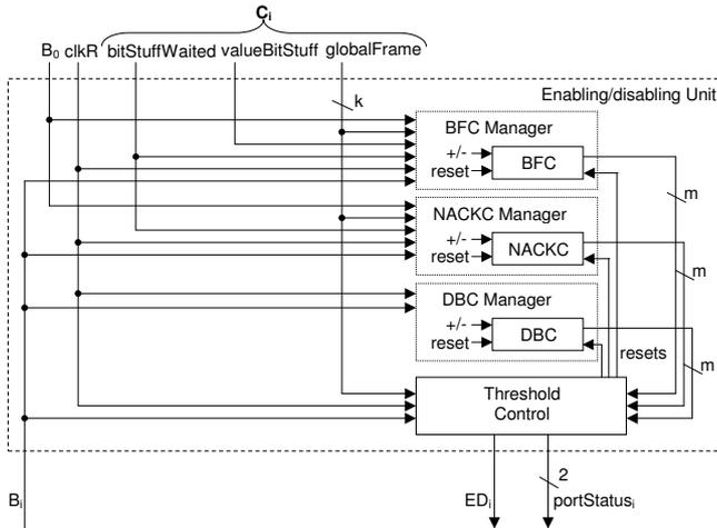
**Figure 5. Internals of the port enabling/disabling Unit**
