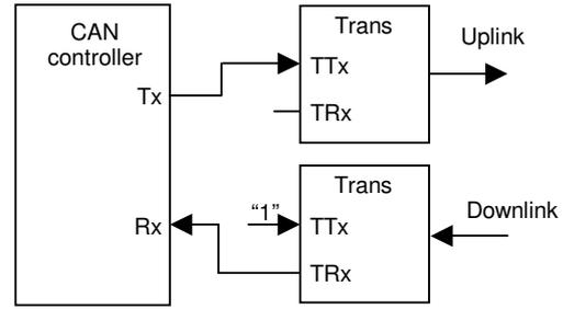
Figure 3. Configuration of the transceivers within one node
