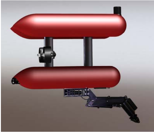
Figure 3. GIRONA500 AUV in intervention configuration.
