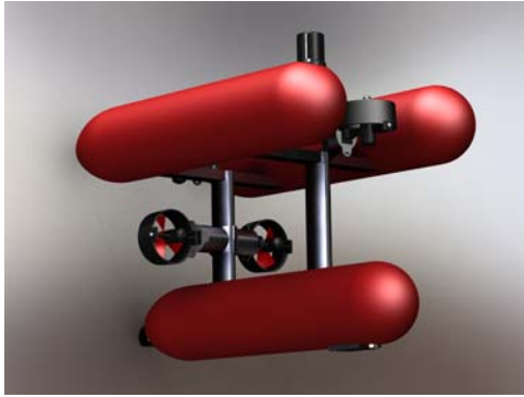
Figure 1. GIRONA500 AUV in survey configuration.
