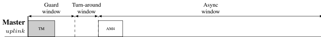
Figure 9: Structure of an Elementary Cycle as seen at the uplink of the Master.
