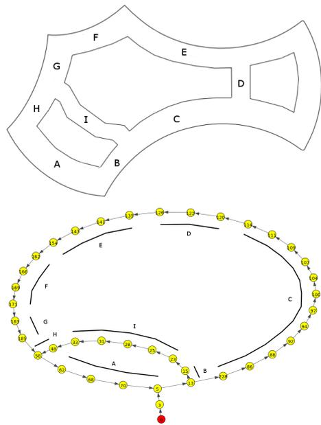
Fig. 4. (Top) Reference map for the Lip6Indoor dataset. (Bottom) Topological map generated using our approach. Each part of the map is identified with a letter in both maps. The red node identifies the beginning of the sequence. Maps locations are visited in the following order: A-B-I-H-A-B-C-D-E-F-G-H-A-B-C-D-E-F-G-H-A-B-I.
