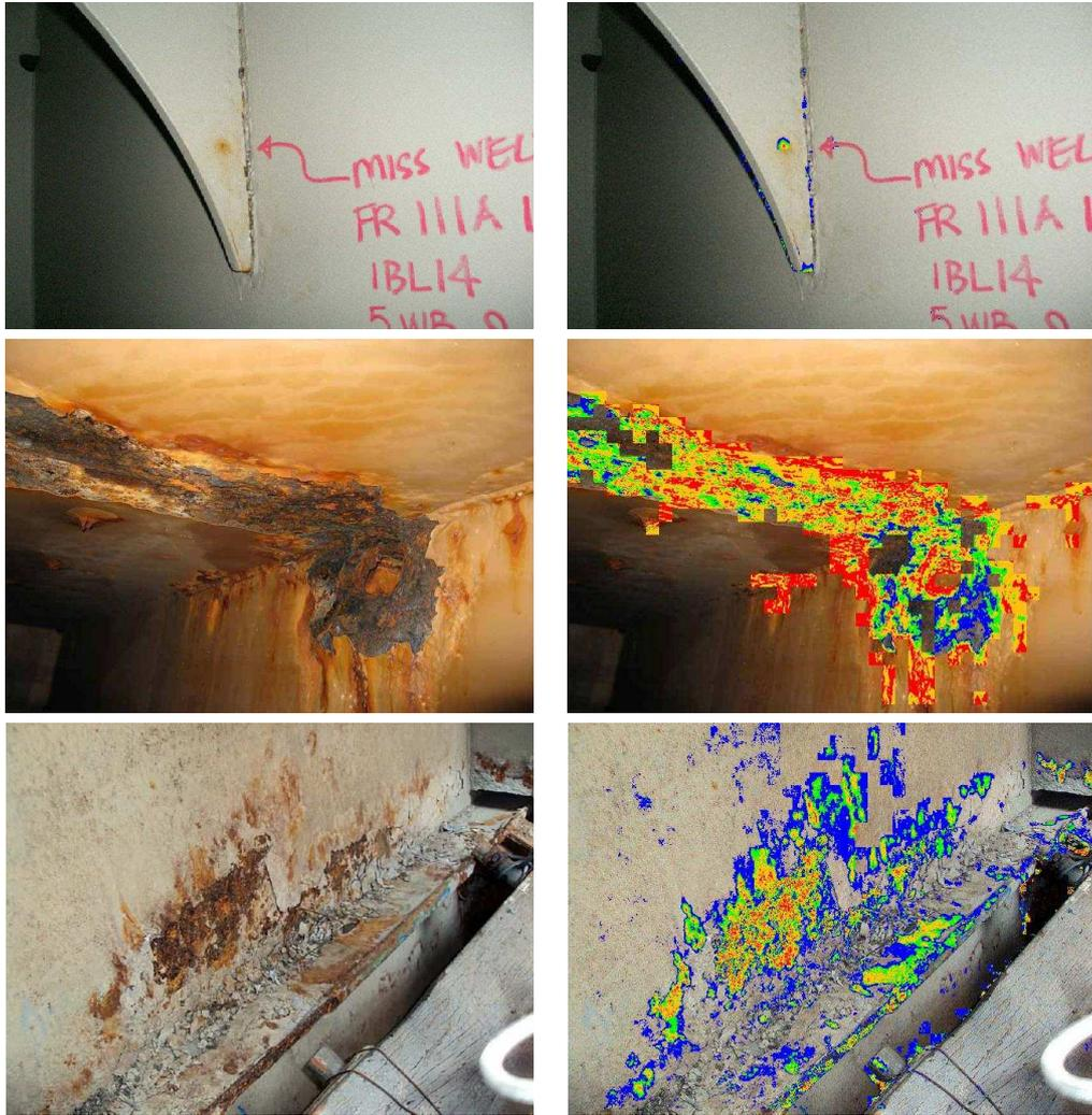
Figure 16: (1st column) Test images and (2nd column) corroded areas detected by WCCD
