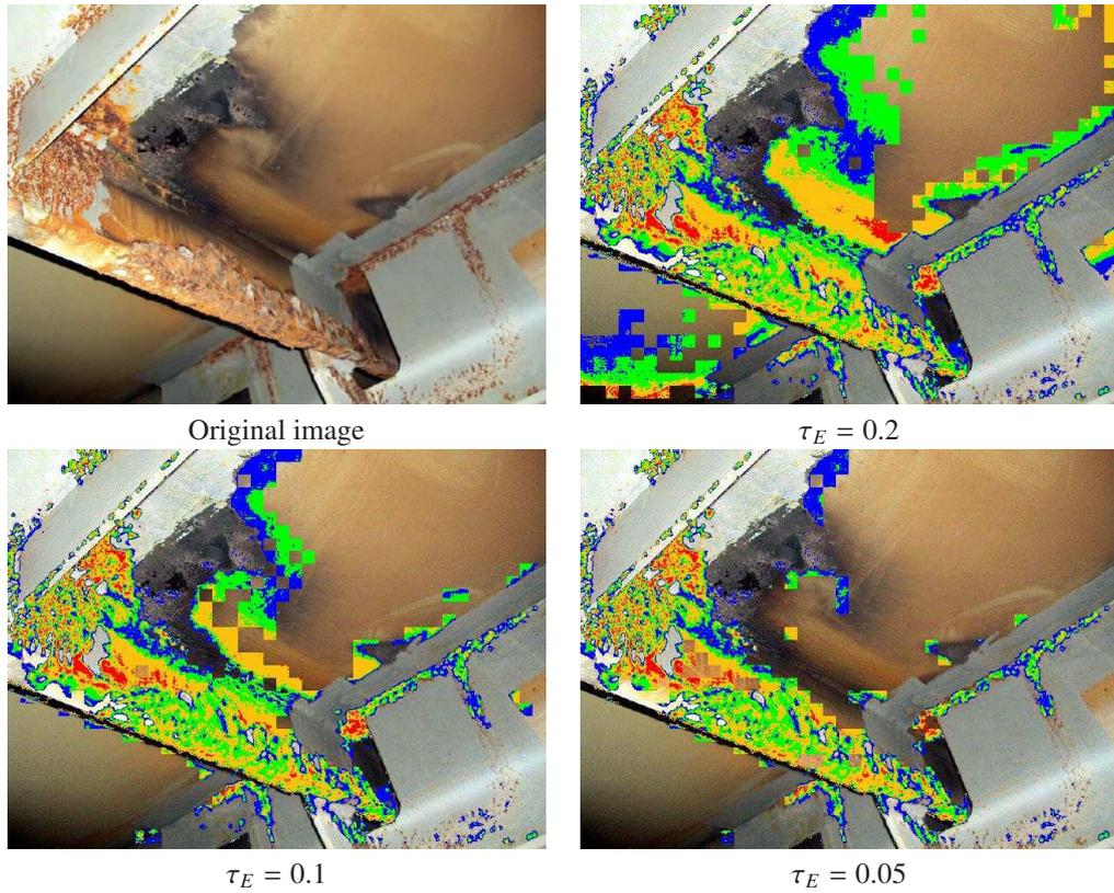
Figure 13: Corroded areas detected by WCCD for different energy threshold values
