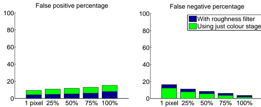
Figure 8: Misclassification percentages with and without the roughness filter (CCD)
