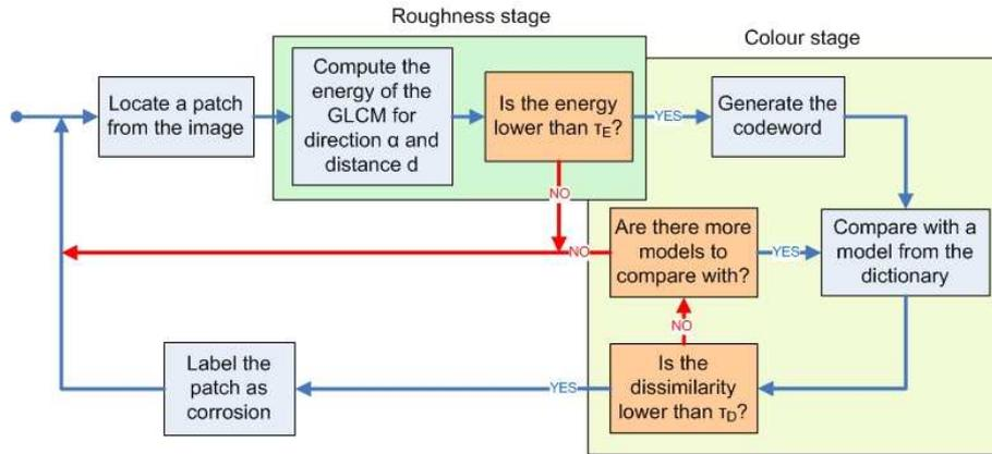
Figure 5: CCD algorithm flowchart
