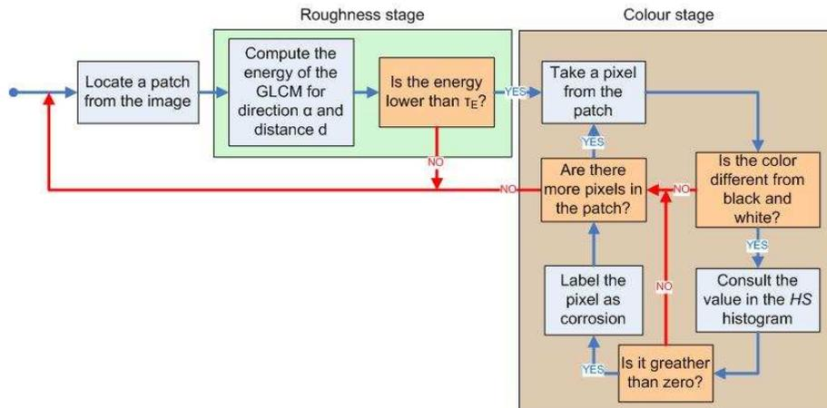
Figure 12: WCCD algorithm flowchart
