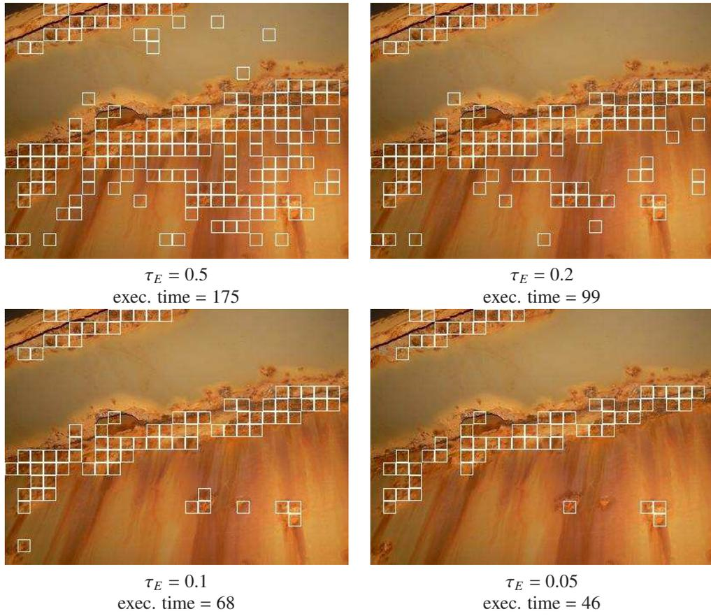
Figure 7: Corroded areas detected by CCD for different  $\tau_E$  values and corresponding processing times (ms)
