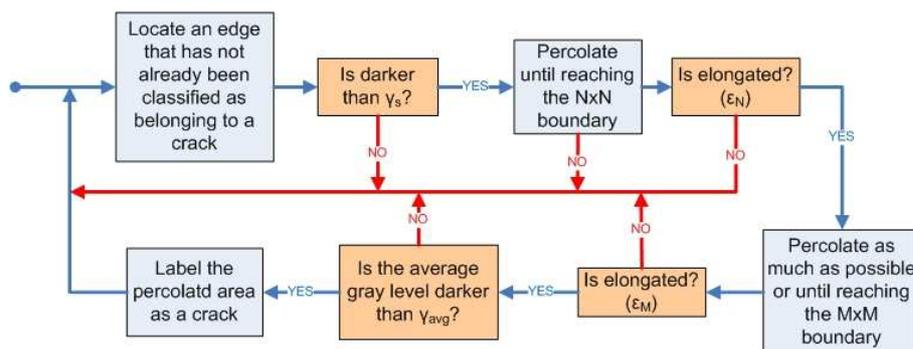
Figure 2: PCD algorithm flowchart
