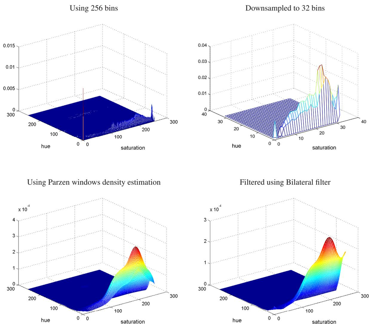
Figure 15: HS histograms resulting from the different filtering strategies (WCCD)
