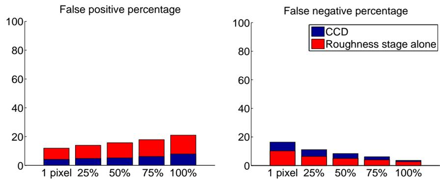
Figure 14: Misclassification percentages for roughness stage in comparison with the ones obtained with CCD
