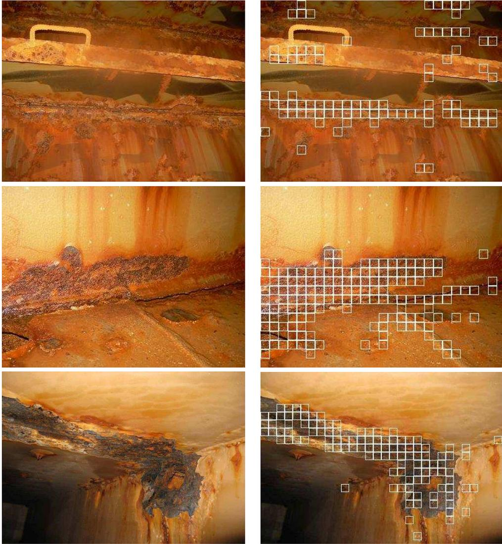
Figure 10: (1st column) Test images and (2nd column) corroded areas detected by CCD
