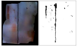
Fig. 9. (left) Mosaic using the images collected by the MAV in a squared trajectory [mosaic contrast has been tuned for visualization purposes]. (right) Defective areas found, shown in black.
