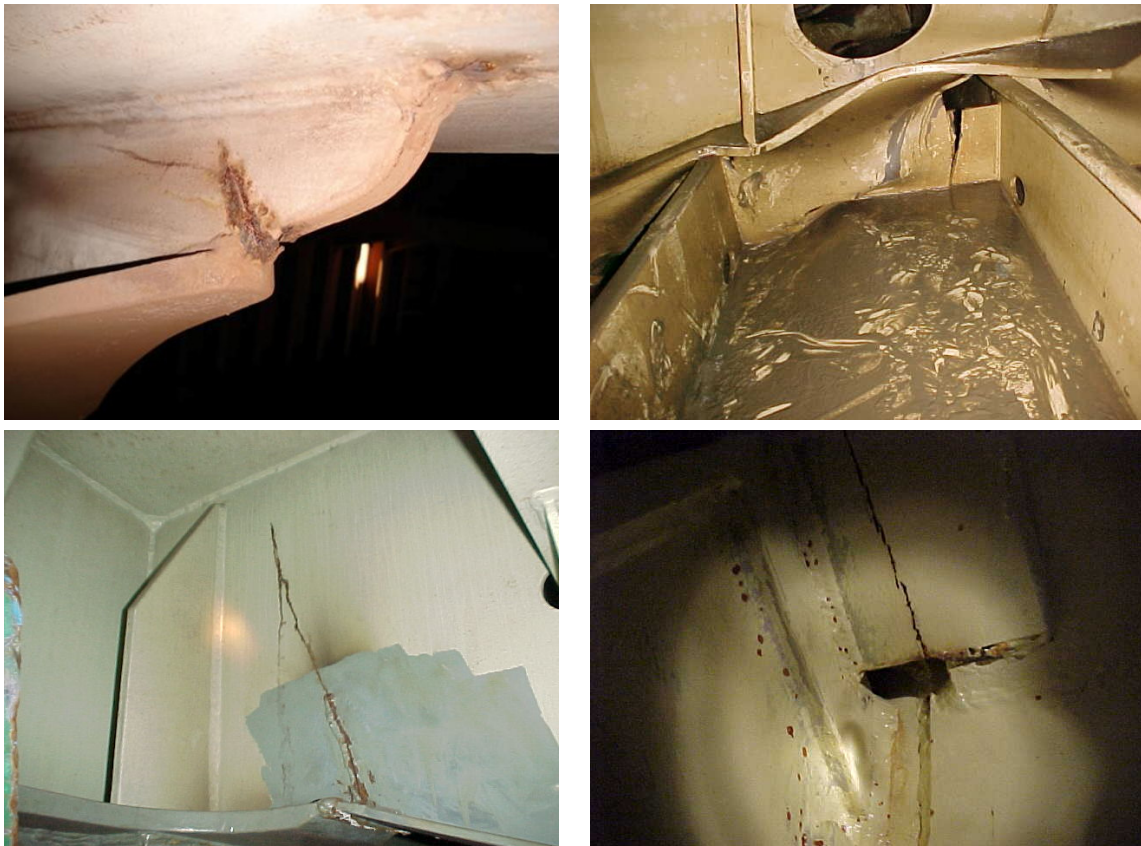
Figure 4.17: Examples of cracks on vessels structures.
