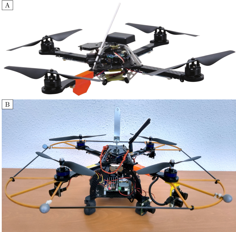
Figure 3.17: The AscTec Hummingbird platform: (A) the aerial platform as delivered by the manufacturer, and (B) the platform equipped with the SS1 and an on-board computer.
