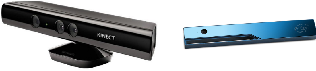
Figure 3.5: RGB-D sensors: (left) Microsoft Kinect and (right) Intel RealSense R200.
