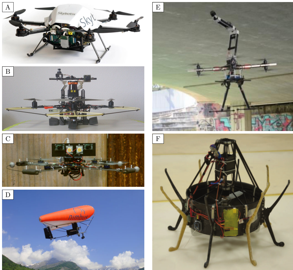
Figure 2.3: Aerial robotic platforms for visual inspection: (A) a hexacopter fitted with the VI-sensor [98], (B) a quadcopter using LiDAR-based SLAM for the visual inspection of vessels [20], (C) a quadcopter fitted with a visual-inertial sensor to inspect boiler systems [97], (D) a hybrid vehicle for the inspection of photovoltaic plants [86], (E) an aerial platform equipped with an arm to inspect structures such as bridges from the underside [108], and (F) a ducted-fan vehicle which allows contact-based inspection [107].
