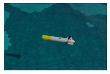
FIGURE 6.3: Screenshot containing a AUV Sparus II in the StoneFish environment
