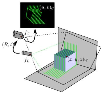
The sensor is formed by a camera and a green laser. In front of the laser, a Diffractive Optical Element (DOE) modifies the beam shape to a set of parallel lines. These lines are projected on the scene and recovered by the camera.
