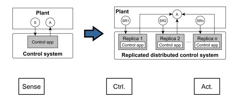
Typical **control applications** cyclically perform **three actions**: sense, control and actuate.
