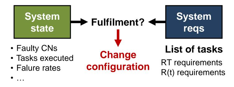
If the system requirements are not fulfilled, the KE decides on the new configuration to apply
